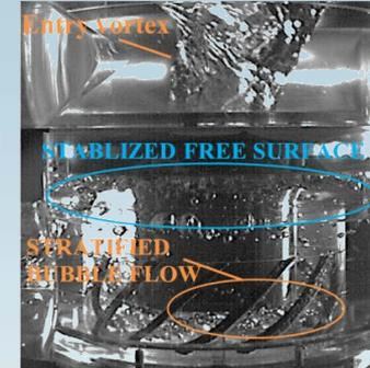
Conceptual flow structures determined from flow images collected from test gullies
